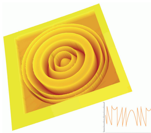
White light interferometry of a diffractive correcting element.
