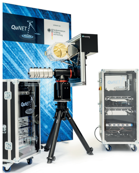
Optical transmitter with a high performance mirror telescope and an entangled photon source for intra-city links (experimental setup).
