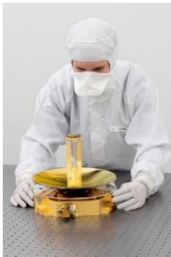
Fig. 1 & 2: A reflecting telescope was developed at Fraunhofer IOF in Jena for the GALA laser altimeter. © Fraunhofer IOF
