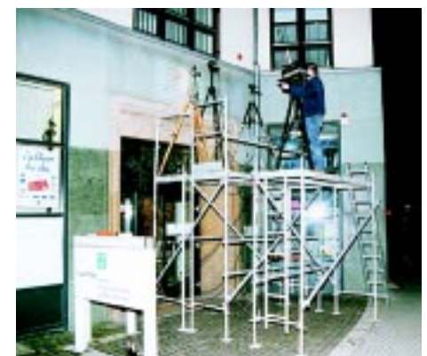
Fig. 3: Mobile camera-fringe projector network while measuring the owl above the entrance of the Fraunhofer IOF.
