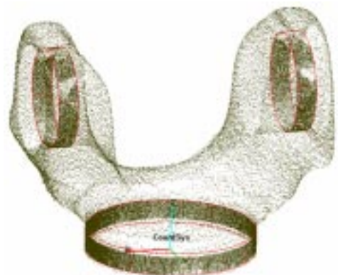
Fig. 9: Point-cloud of an automotive part measured with kolibri.
